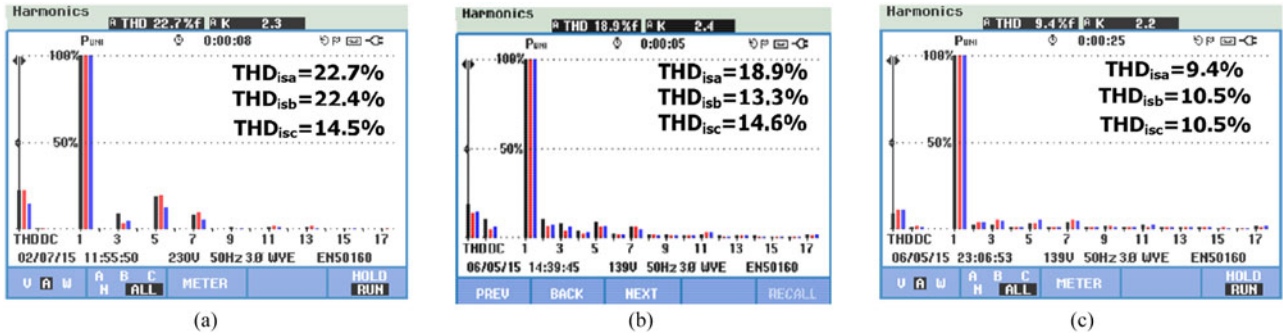
Fig. 11. Experimental source current spectrums: (a) Before compensation, (b) after the state-of-the-art control method compensation [22], and (c) after the proposed control method compensation.
